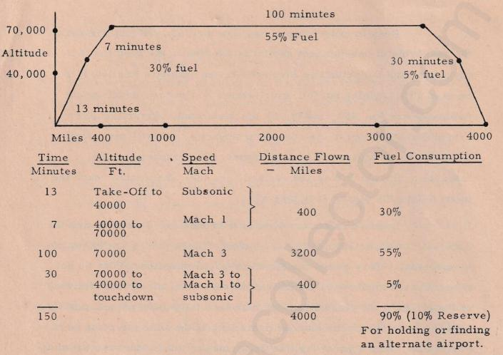
13 minutes after take-off, it climbs to an altitude of 40,000 ft. reaching the speed of Mach 1 without fear of sonic boom effects. In the next 7 minutes, it accelerates to 70,000 ft. The elapsed time from take-off to cruise altitude is 20 minutes; distance travelled is 400 miles; fuel consumed is 30%.
