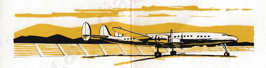
Before entering the main take-off runway, a stop is made at the "run-up" area where engines and propellers are given a final functional check. All control surfaces are operated. The crew completes the last of sixty-nine pre-flight inspections by testing the electrical, electronic, pneumatic and hydraulic systems. When certain that all controls and instruments are functioning properly, the pilot radios the control tower, identifies the aircraft and requests permission to take off.
