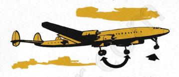
A slight thump can be heard inside the airplane as the tricycle landing gear is extended and locked into position. Seconds later, flaps begin to extend from the trailing edge of the wings, accompanied by the humming sound of hydraulic cylinders being actuated. These flaps give the Super Constellation more "lift," permitting it to land more slowly.
